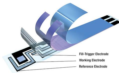
Figure 1. Example diagram of a blood glucose test strip from Abbott [1].
