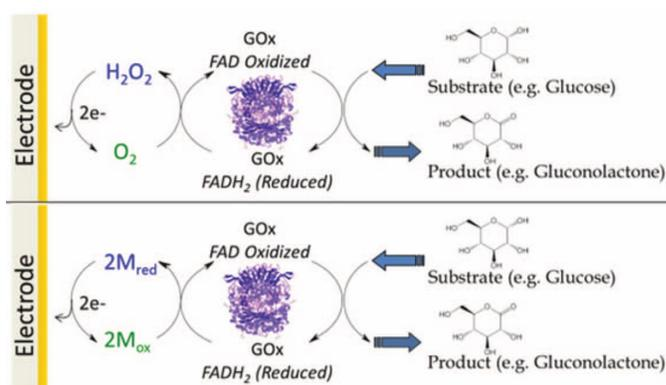
Figure 2. Comparison between the reaction of the first generation amperometric biosensors ( $H_2O_2$  sensing) and the second generation biosensors (with a mediator). GOx: glucose oxidase; FAD/FADH<sub>2</sub> flavin adenine dinucleotide (enzyme's cofactor) M: mediator. Image adapted from [18]
